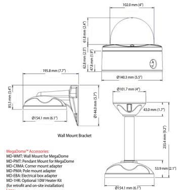
Integrated 4.5-10mm IR corrected Megapixel Varifocal Lens (AVxx55 models) Ø - Diameter Integrated 8-16mm IR corrected Megapixel Varifocal Lens (AVxx55-16 models) Pendant Mount Bracket
